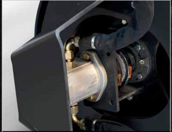
The hydraulic motor is coupled to an eccentric shaft which creates the required vibration.
