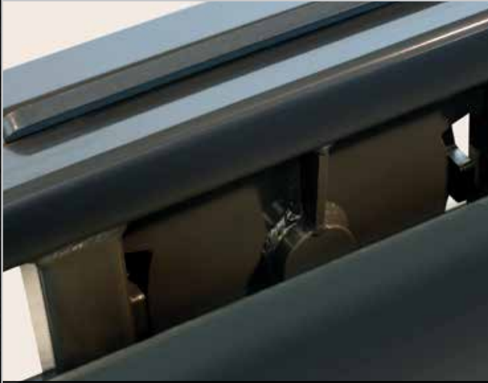
Free drum oscillation keeps more of the drum in contact with the surface on uneven terrain - up to 15°
