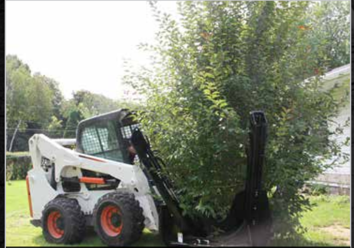
Overlapping blades ensure a clean cut and support of the root ball.
