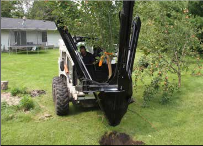
This Tree Spade has full hydraulic controls for in-cab operation and is fully adjustable to fit most skid steers.
