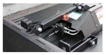
Adjustable stabilizer bar prevents deck flexing while allowing the operator to control the front of the deck height to the operator's preferred height.
