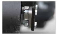
Stainless steel greaseable bearing and 8" roller allows mower to stay in contact with cutting surface providing smooth ride for operator.
