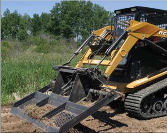
Use back or front edge for back dragging and leveling of surface.
